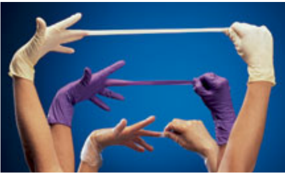
Glove materials have different stretch capabilities. This difference can affect in-use barrier performance. Glove materials from top to bottom: Natural Rubber Latex, Nitrile, Vinyl.
